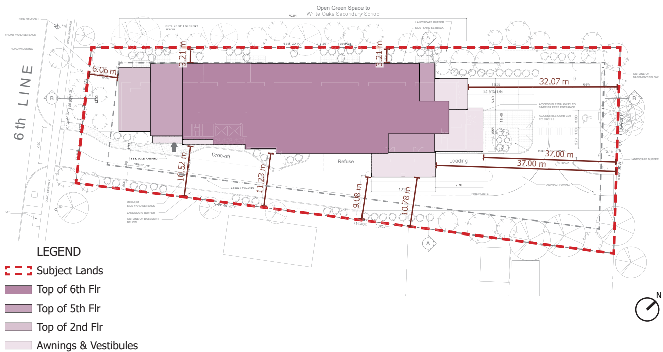
Figure 7.1 : Building Placement and Setbacks
