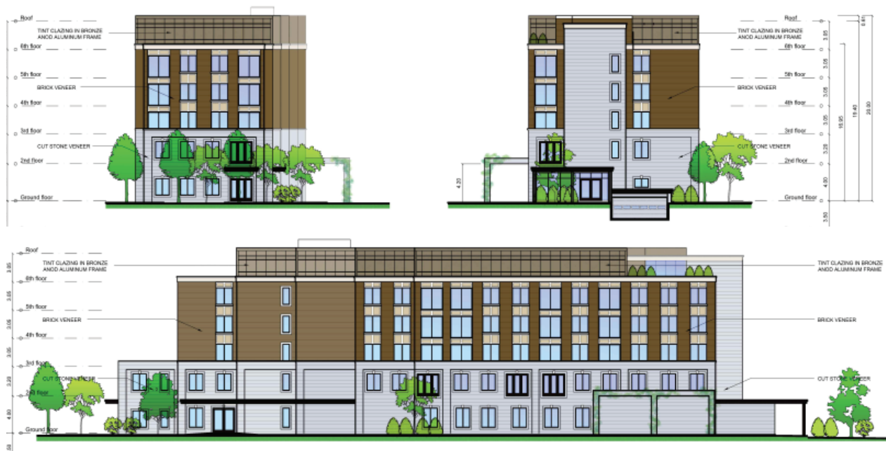
Figure 7.8 : West, east and south elevations
