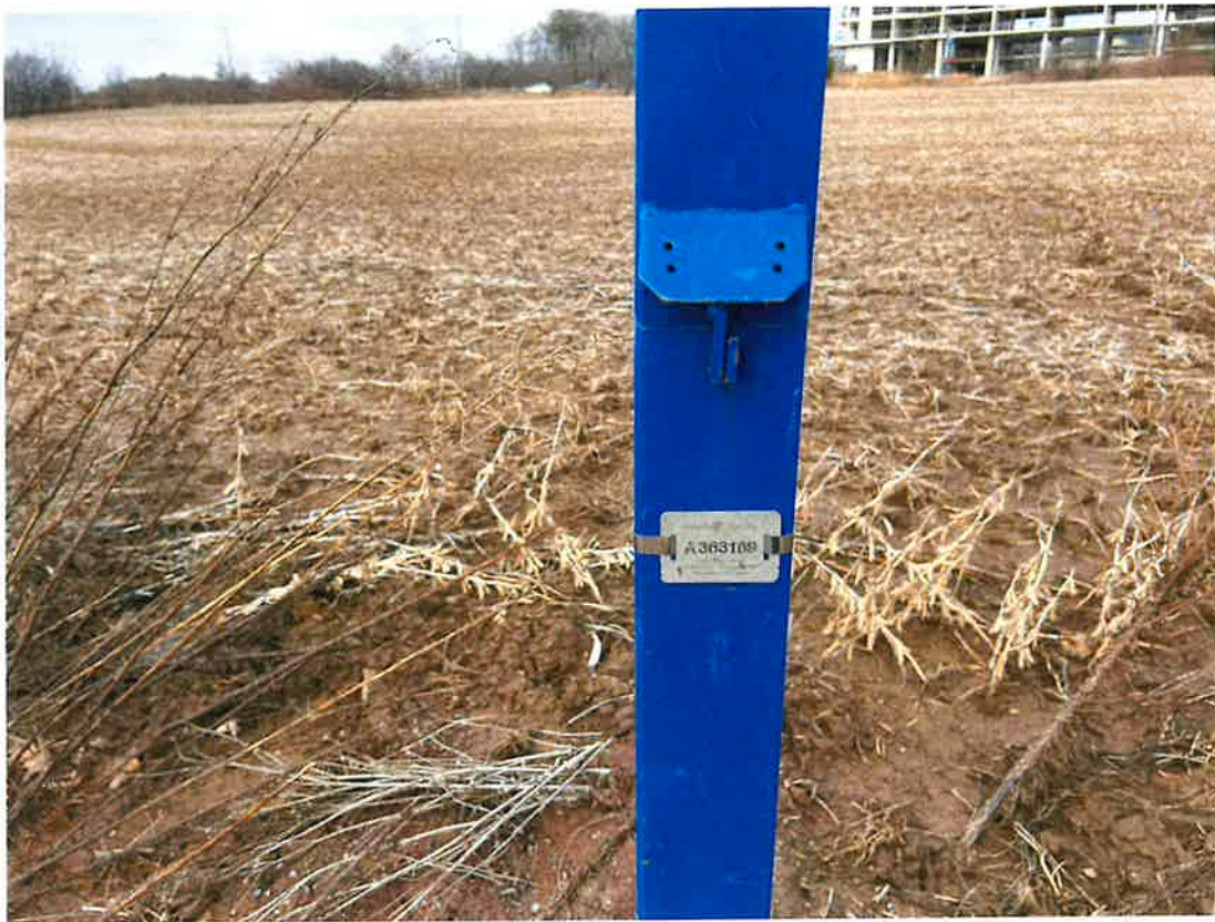
Close up view of monitoring well located on eastern portion of subject site.
