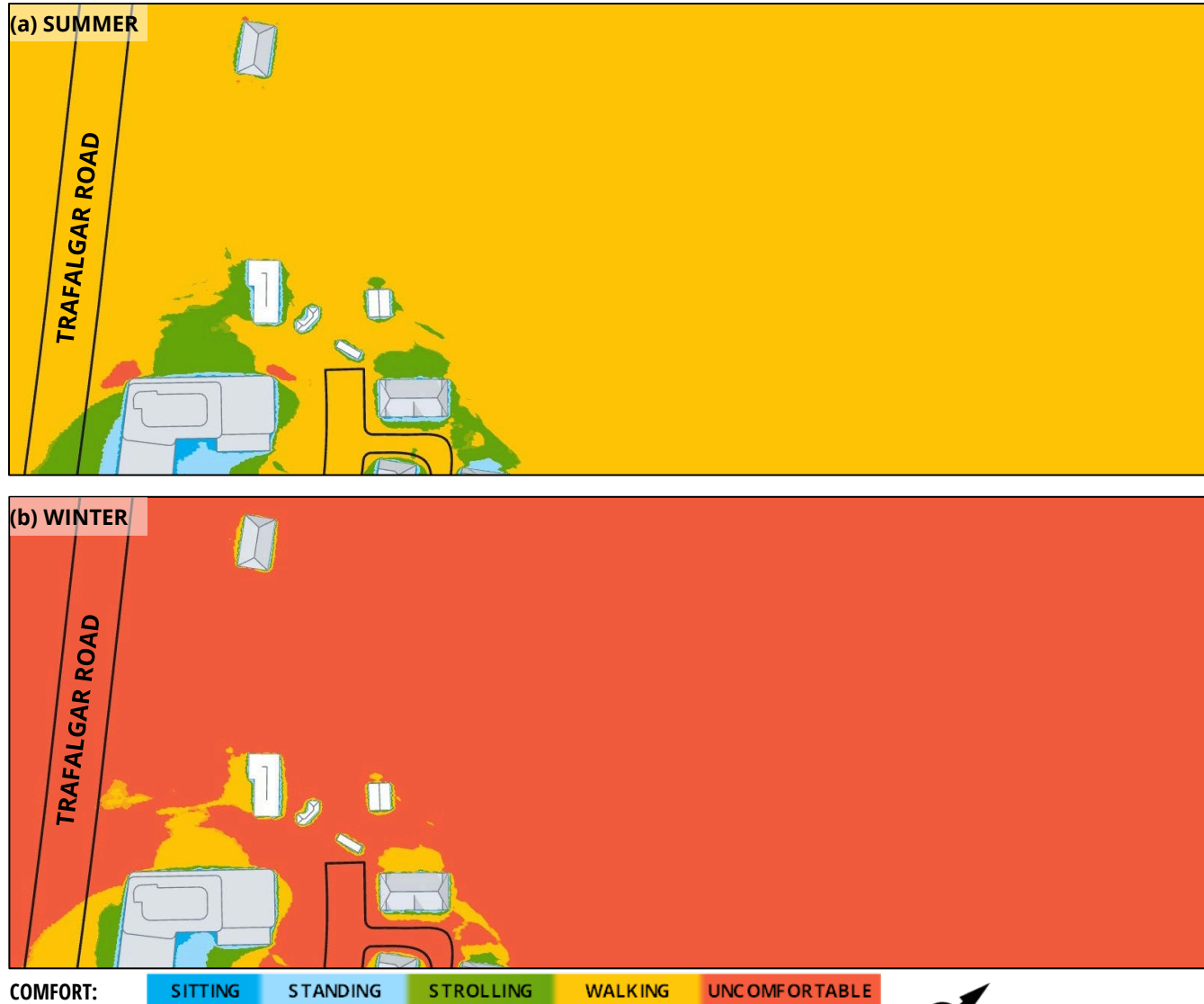
Image 8: Predicted Wind Conditions – Ground Level – Existing Scenario
