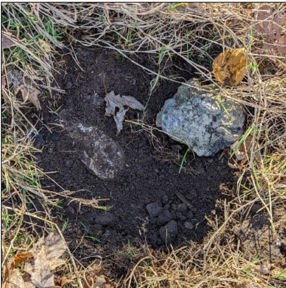
Image 19 : Test Pit showing disturbed soils and concrete debris.
