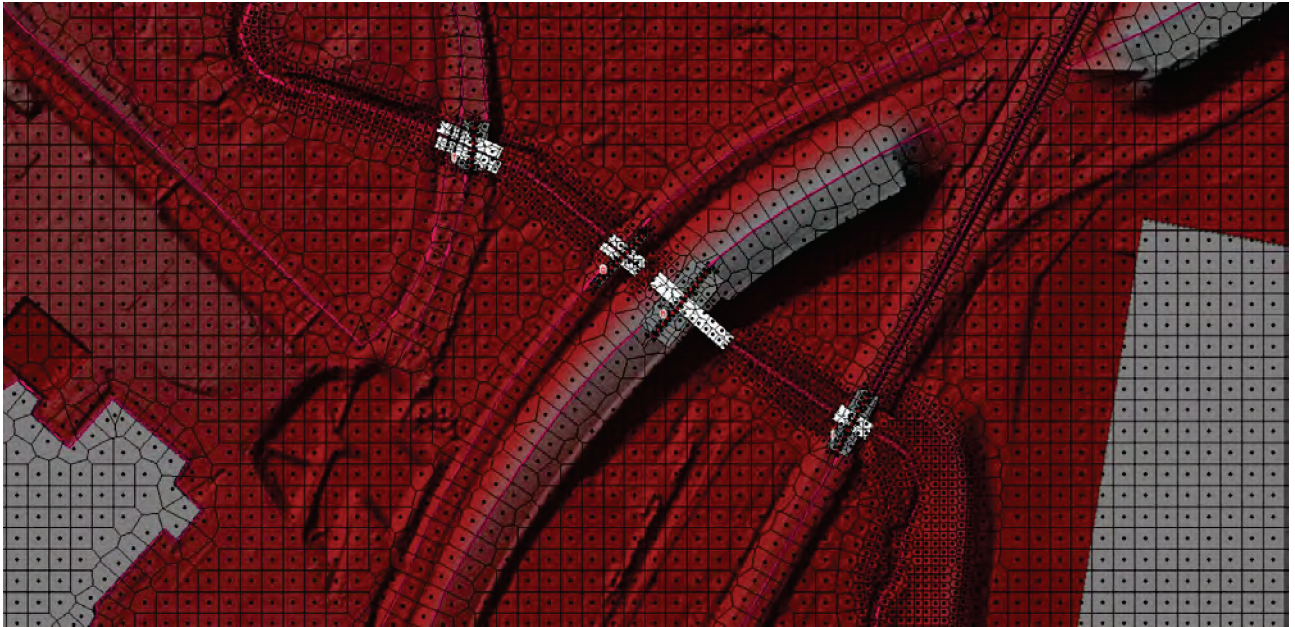
Figure 3.1 Computational Mesh of the 2D Study Area
