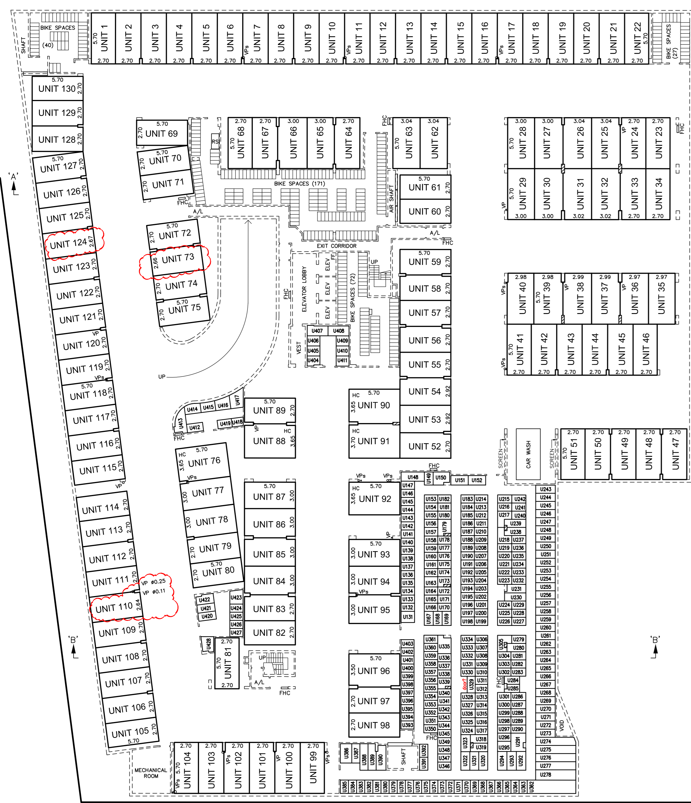
PLAN VIEW ILLUSTRATING UNITS 1 TO 130 INCLUSIVE (Residential Parking, Includes 5 Accessible), UNITS 131 TO 428 INCLUSIVE (Storage), 310 Residential Bicycle Spaces, LEVEL B
