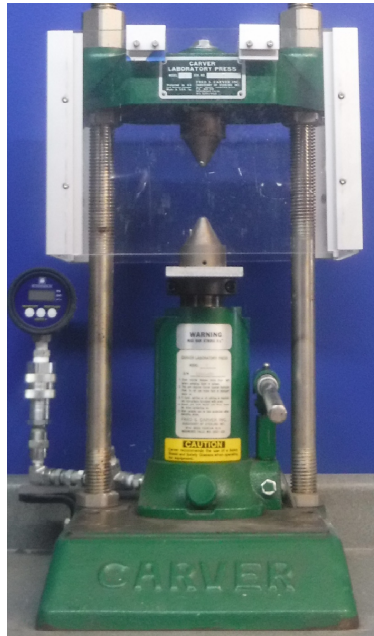
Figure 2: Point load tester equipped with digital pressure gauge.
