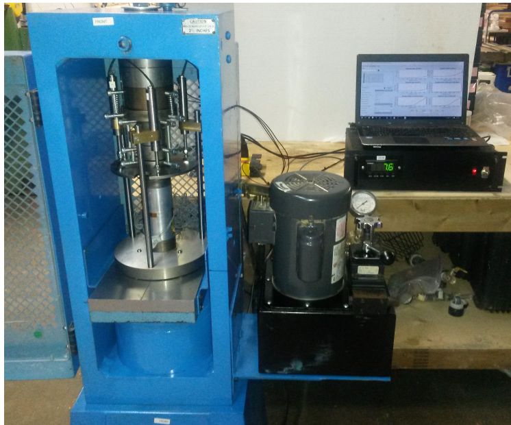
Figure 1: Forney loading frame setup for UCS testing.
