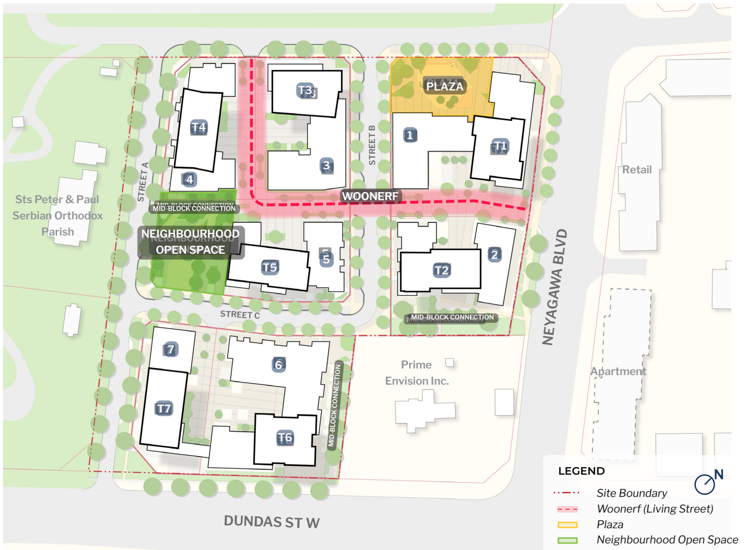
Figure 13. Site Organization: The site is organized around a new network of public streets and served by a pedestrian friendly woonerf
