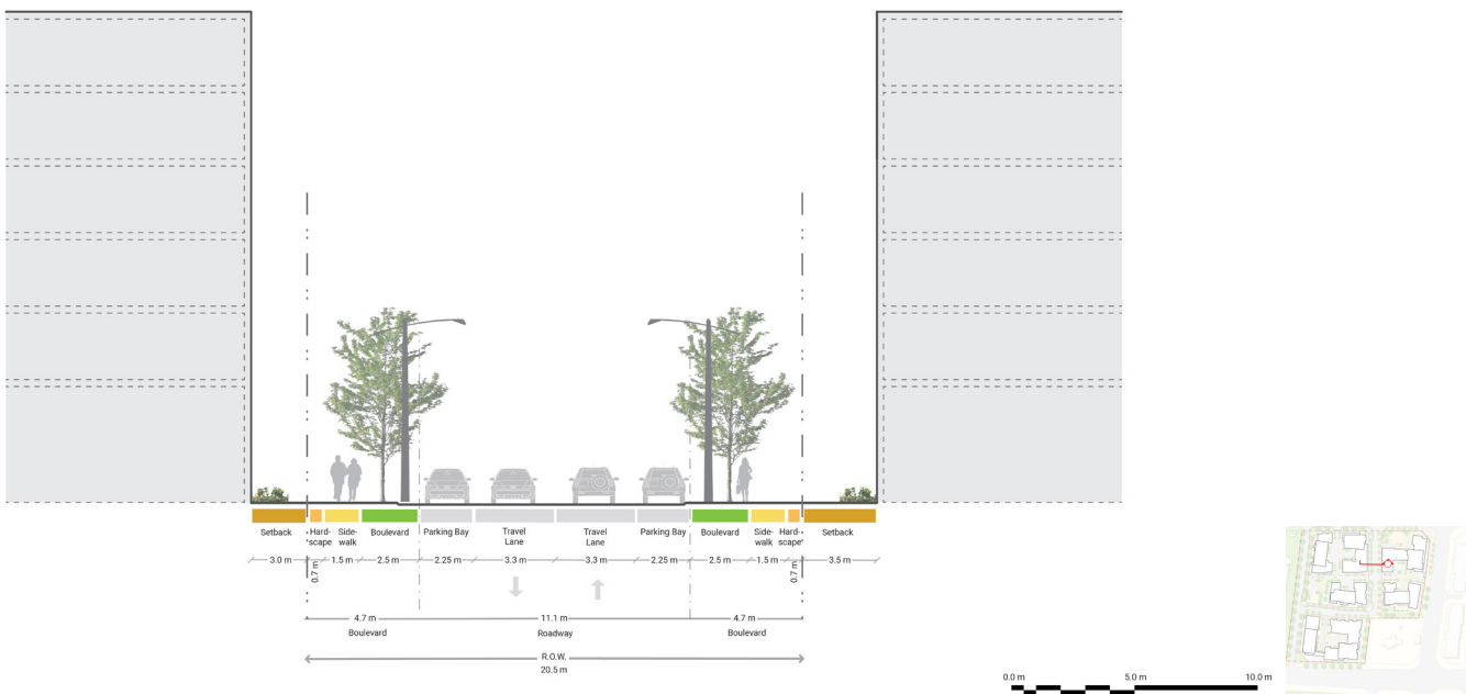
Figure 27. Cross Section of Street B
