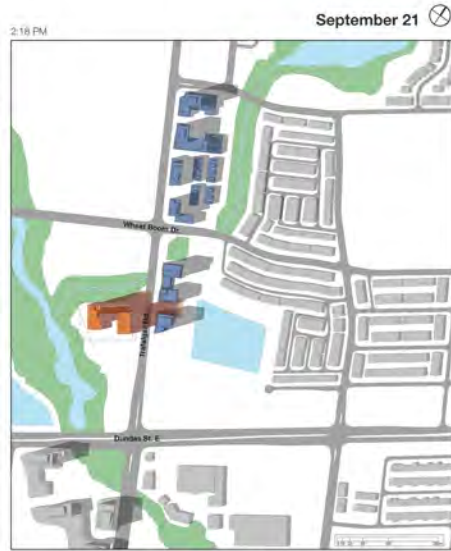
Proposed / Under Construction Context: 3060 & 3068 Trafalgar Rd. 33 Storeys Shadow Existing Context: 3060 & 3068 Trafalgar Rd. 30 Storeys Shadow 3060 & 3068 Trafalgar Rd Property Line: 3060 & 3068 Trafalgar Rd. Proposed Development Shadow Studies
