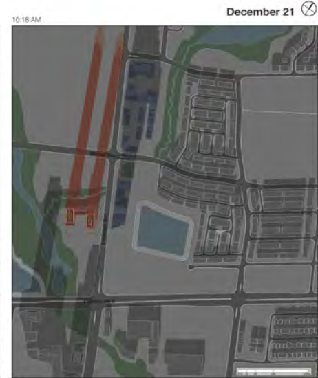
Proposed / Under Construction Context: 3060 & 3068 Trafalgar Rd. 33 Storeys Shadow Existing Context: 3060 & 3068 Trafalgar Rd. 30 Storeys Shadow 3060 & 3068 Trafalgar Rd Property Line: 3060 & 3068 Trafalgar Rd. Proposed Development Shadow Studies
