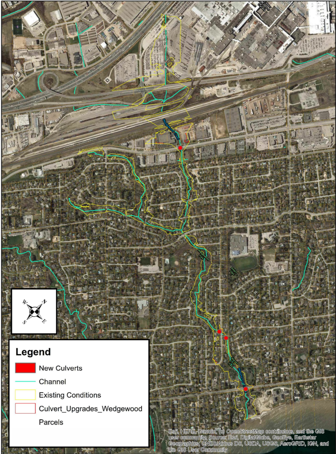
Figure 5.16 Comparison of Floodlines Between Existing Conditions and Preferred Alternative for Lower Wedgewood Creek
