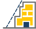
ANGULAR PLANE A geometric measurement that maintains solar access and height transition
