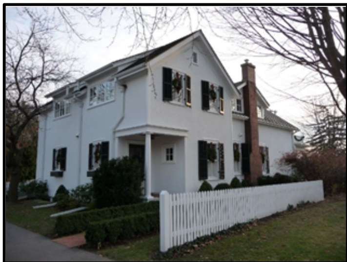
Figure 60: 53 Navy Street (left) – addition to rear and visible from William Street. Height of addition matches; consistency in gable roof form stucco cladding and public facing style of windows/doors and trim
